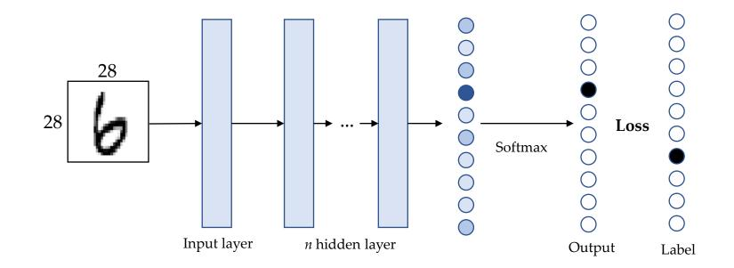
One of the most used functions for multi-class classification is **cross-entropy loss**, defined as:
