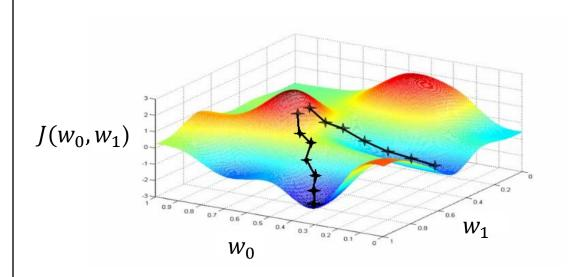
In the beginning, the line has random  $w_0$  and  $w_1$ . **Gradient descent** moves the point (by updating the values of  $w_0$  and  $w_1$ ) in the direction where the **Loss** function decrease.
