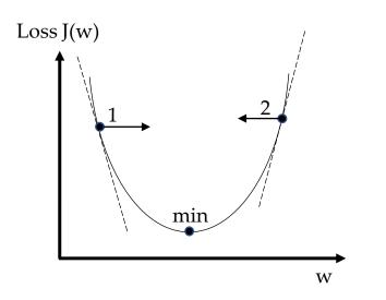
Backpropagation is the technique that allows to compute the derivative of the loss with respect to the parameters. **Optimization**: we want to find the value of w which minimizes J(w). To do this, we will update w at each step by the quantity:
