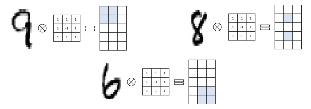
In CNN, these filters are not hardcoded as in this example but learned during training
