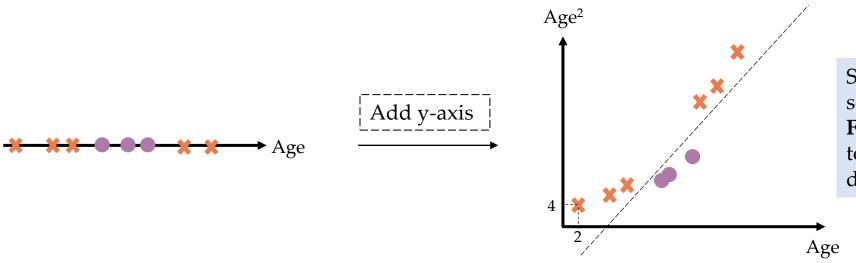
Support Vector Machines use something called **Kernel Functions** that we can be used to *systematically* find higher dimensions' axis
