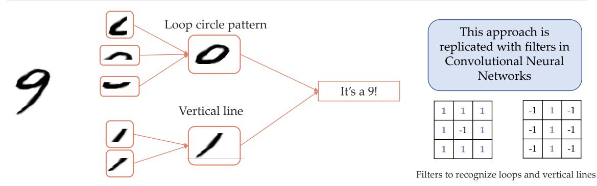
A CNN is an algorithm that can take in an input image and apply filters that, during training, learn to distinguish various aspects/objects in the image
